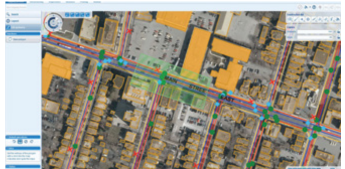
With GeoMedia Smart Client, field engineers can map a location for a new digging permit.
